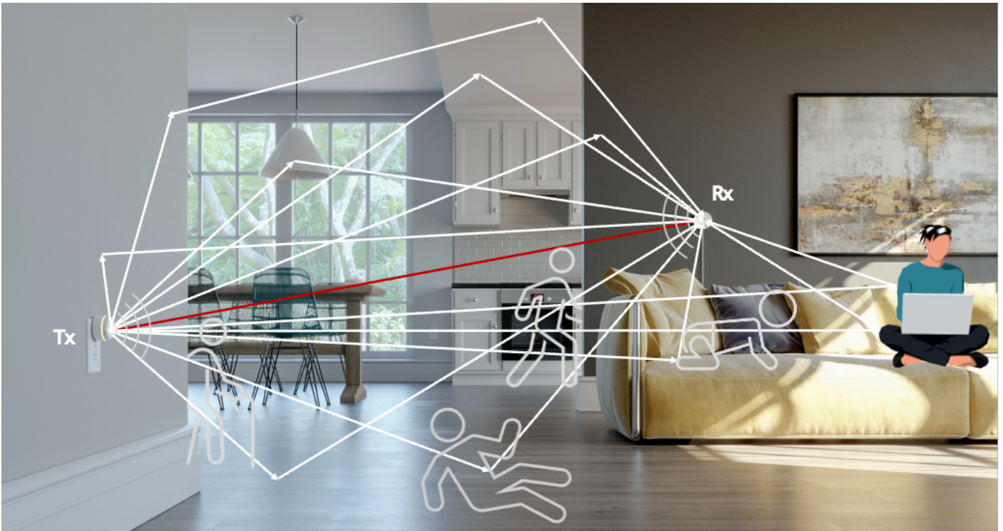
Fig. 1. An illustration of multipath propagation of WiFi signals in indoor space. Human activities at different locations altering the propagation can be sensed from the received signals.
